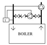
To eliminate totally the problem, it should make perfect the above mentioned design to maintaining the temperature of the boiler (55  $^{\circ}$ C) also by night and add a further temperature limit fuse thermostat tha operate to the unit mixer valve not forward to the boiler, water not at 55  $^{\circ}$ C.
